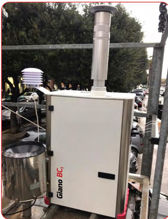
Developed in partnership with company PM\_10, a University of Genova - Department of Physics spin-off, **Giano BC<sub>1</sub>** can evaluate the Black Carbon component collected on the filter thanks to optical module measuring the laser beam reflectance.
