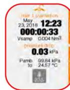
Thanks to a simple and intuitive interface, **1PMxHV** can be quickly programmed with date and time of start of sampling, duration and cycle of the sample and number of cycles.
