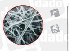
Those filters are made of high purity borosilicate fibers. Glass fibers filters became, during the last 20 years, the most diffused filtering elements for stack emission and ambient sampling thanks to their low cost but also because of the quality improvement granting better resistance and easier to handle.
