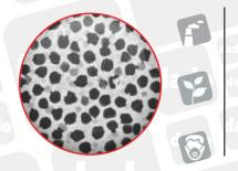
Those membranes are made of anodized alumina and allow effcient separations with low pressure drops. Completely organic free, those membranes grant a very low adsorbing grade during the sampling operation. Max application temperature is 400°C
